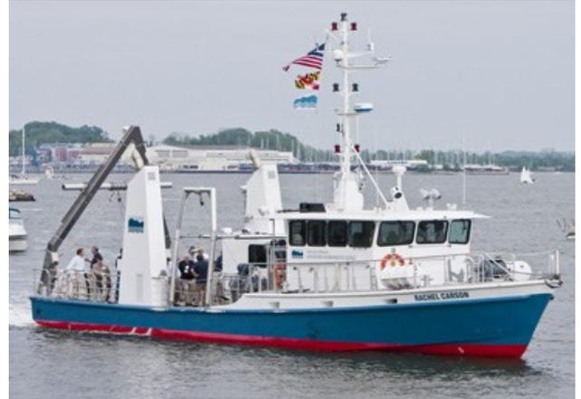
The *Carson* has been used to collect water quality samples; to tow plankton nets; to conduct box coring operations; to deploy a data buoy; to ground truth aircraft deployed instruments and as a platform to teach undergraduate and graduate students estuarine sampling techniques.
